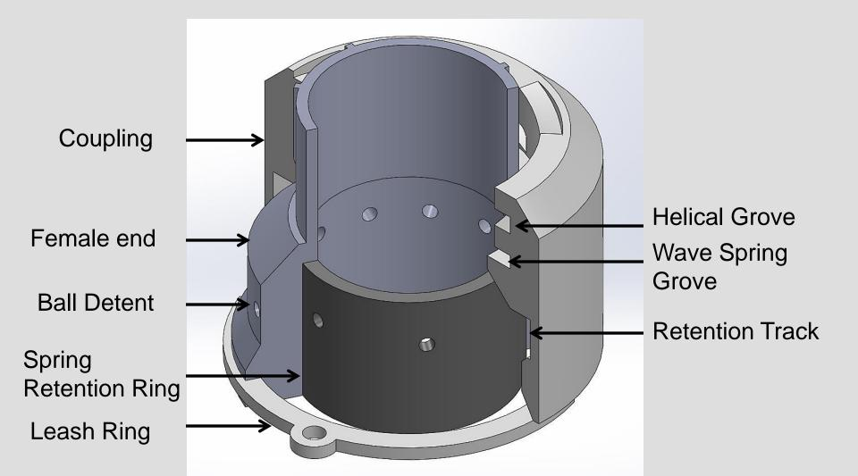
Metal Prototype (Exploded View)
